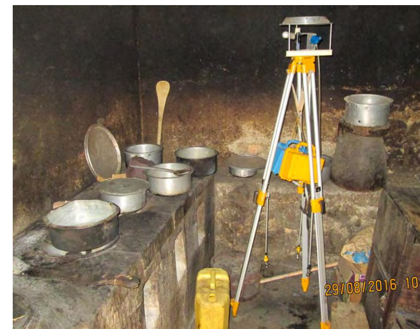
Fig. 4: Monitoring HAP in a traditional cookstove kitchen during baseline
