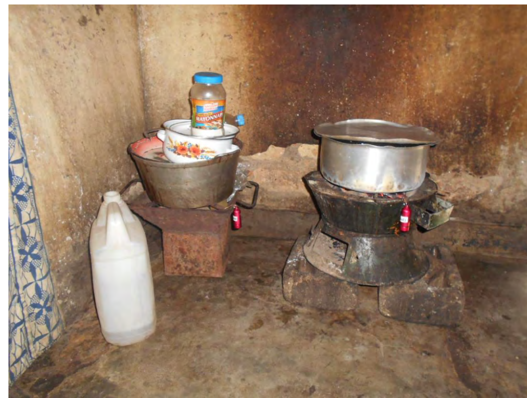
Fig. 1: Traditional charcoal cookstoves in a kitchen. The red cylinders attached to the stoves are temperature data loggers that serve as stove use monitors.
