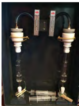
Mist chamber devices used in sampling →
